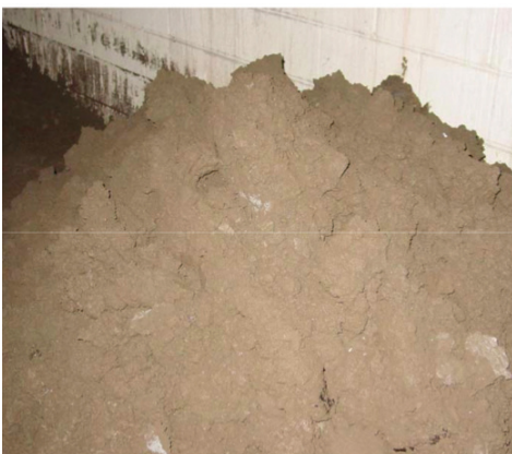
Final clean processed product of about 55 percent solids, ready to be transported for beneficial use on the golf course.
